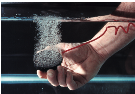
Figure 4: Submersed underwater with 60 psi input pressure, 3 SCFH bleeds evenly out of the face of a 2.5-inch diameter New Way porous bearing. This bearing carries 150 lbs. of load at 0.0002-inch air gap.
