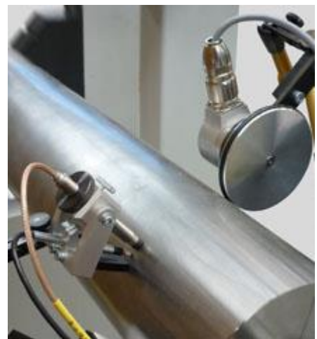
Runout testing, mechanical, electrical, and total (flexible shaft shown)
