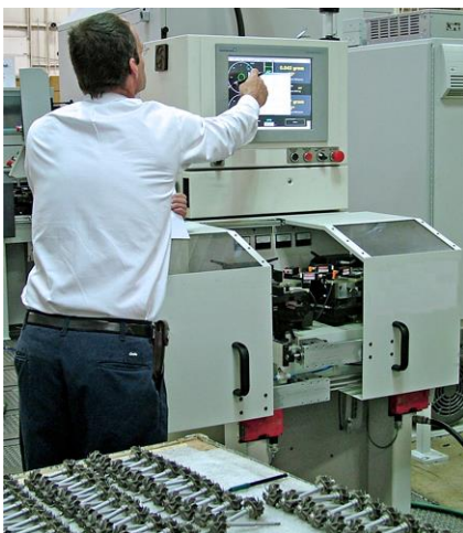
Small rotors, vertical up to 150 lb (68 kg) (wheel and shaft assemblies shown)
