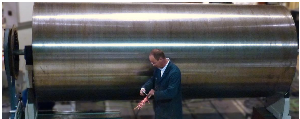
Large horizontal rotors up to 15,000 lb (6800 kg) (5-ton rotor shown)
